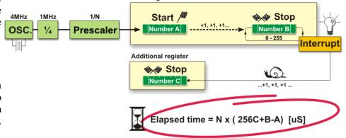
Meaning that in order to generate one pulse on its output, it is necessary to bring 1, 2, 4 or more pulses to its input. One such circuit is built in the microcontroller and its division rate can be changed from within the program. It is used when it is necessary to measure longer periods of time.
